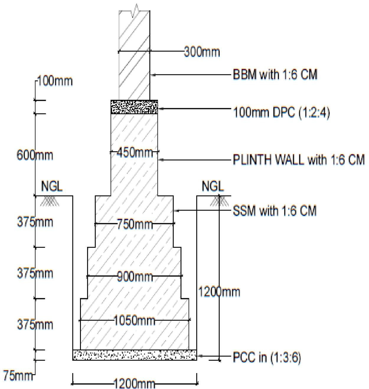
CROSS SECTION OF SIZE STONE MASONRY
