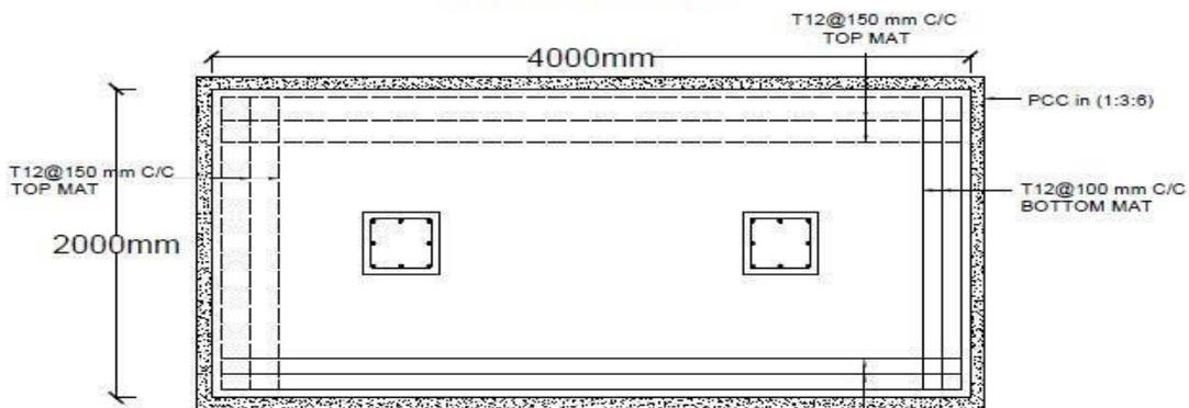
PLAN SHOWING REINFORCEMENT DETAILS OF COMBINED FOOTING
