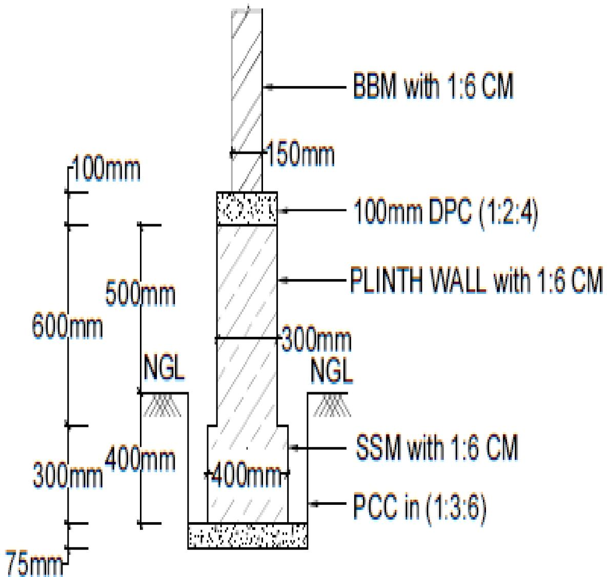
**CROSS SECTION OF SIZE STONE MASONRY
